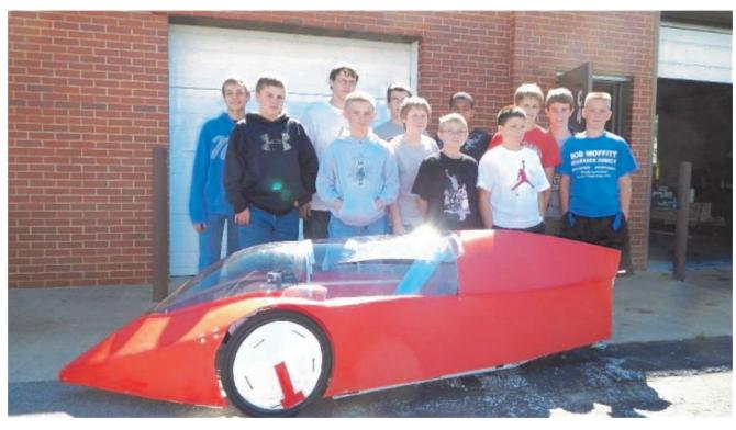
The single-seat car weighs about 100 pounds and is powered by a 1.3 hp 35 cc Robin/Subaru motor that is typically used on motorized bicycles. A custom two-speed gearbox was built for
