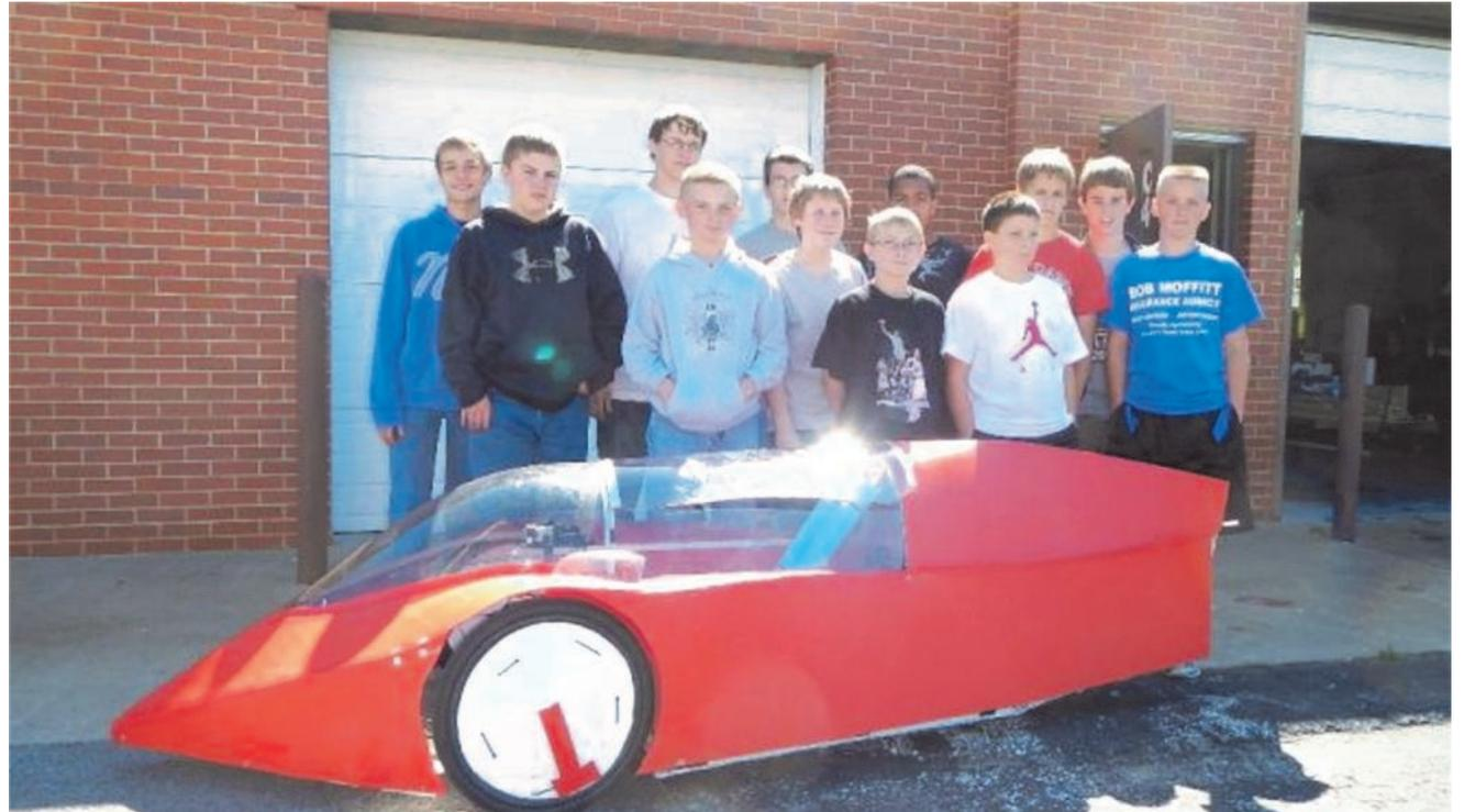
The single-seat car weighs about 100 pounds and is powered by a 1.3 hp 35 cc Robin/Subaru motor that is typically used on motorized bicycles. A custom two-speed gearbox was built for the car and its streamlined corrugated plastic bodywork designed using scale models shaped in a small wind tunnel at the school.
