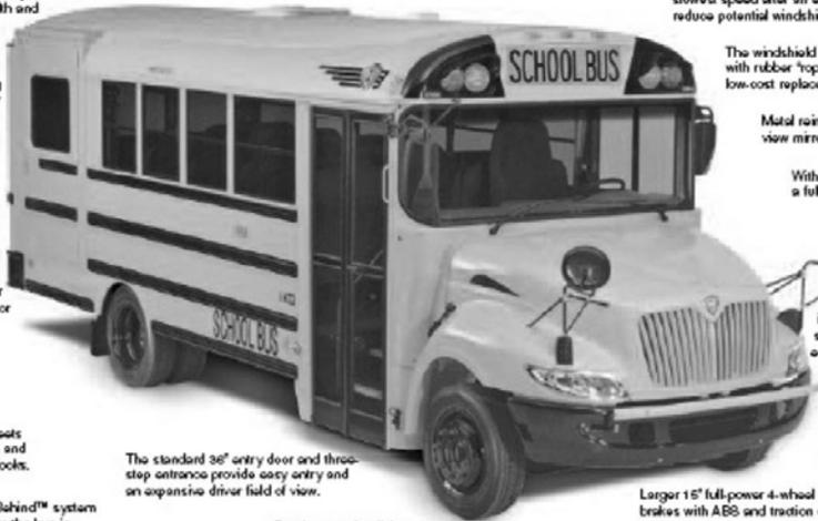
The standard 36" entry door and three-step entrance provide easy entry and an expansive driver field of view.
